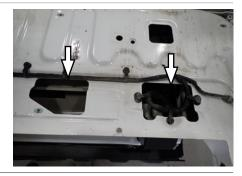
Use a pry tool to remove the push fasteners securing the factory harness to the tailgate. Route the custom wiring harness down inside the channel of the hinge with the factory wiring.
