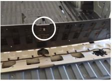
Open the multipro tailgate step/bed extender. Use a trim tool to remove the two square filler caps on the passenger side, being careful to not dent or scratch them.
